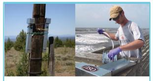
(On the left) Samplers strapped to a fence post. (On the right) An OSU researcher loads an air sampler with the passive sampling material.
